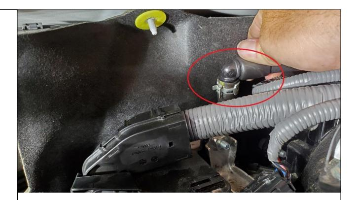
The hose with the short rubber section will connect to the intake manifold fitting, be sure to preinstall the hose clamp and ensure the screw of the clamp is on the upward side of the hose to allow for easier tightening of this clamp. Tighten clamp and pull-on hose to ensure it's tight enough to not pull off, the intake manifold is pressurized by the turbo's so this needs to be tight enough to withstand the pressure!
